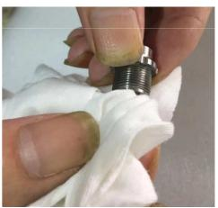
3). Apply appropriate Lubricant on the thread  $\circ$
